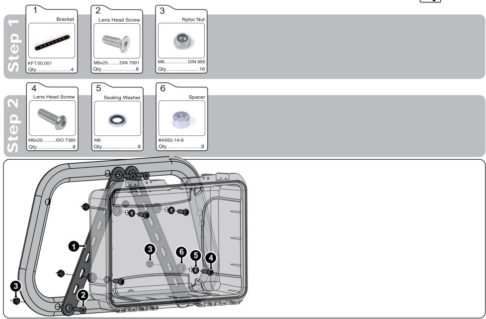
**Step One:** Bolt the mountings bracket to the rack using the included hardware.
