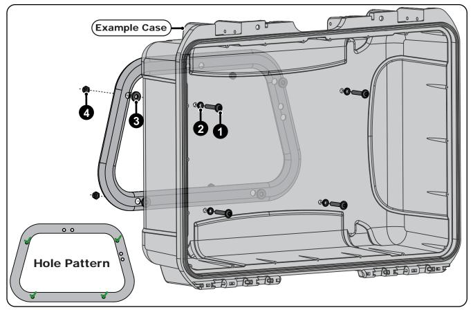
**Step One:** Place the side carrier on the back of the luggage case and mark the hole pattern on the case. Using a 6mm drill bit, drill all four holes through the back side of the case.
