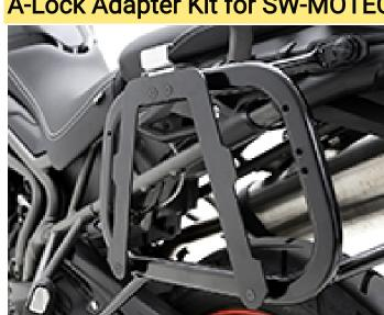
DrySpec A-Lock Side Case Adapter Kit for SW-MOTECH EVO / PRO & most GIVI PL series side carriers is required to mount a set of H35 cases to your luggage rack. The wedge shape design of these frames provide solid and secure mounting that can be done with one hand.
