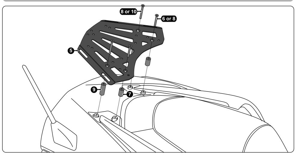
**Step Three:** With the rack brackets bolted in place reinstall the rear center top cover plastics, grab rails and seat. Use the supplied spacers to level the rack, then bolt the steel rack to the brackets. (If installing with OEM backrest use the longer bolts to attach the steel rack to the brackets)
