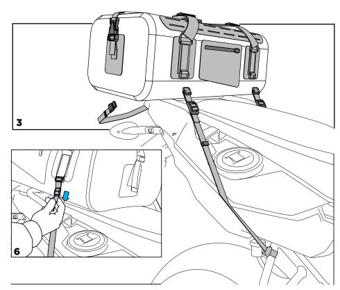
**Step Three:** Note: In many situations, the dual ended slip-lock strap is easier to use in place of the regular slip-lock straps on the rear. It creates a closed loop that can be passed under a license plate bracket or tail light assembly.
