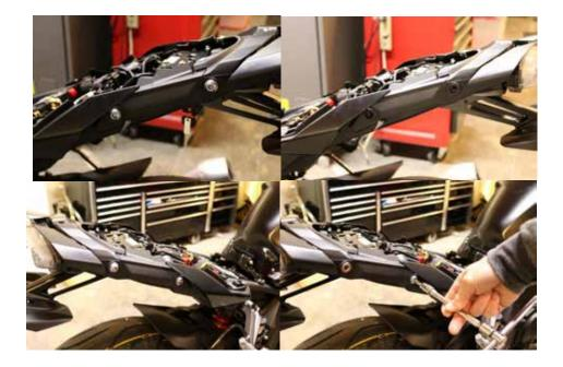
4. Remove the tail light cover screws. Remove the tail light cover.
