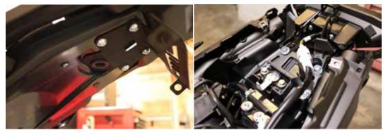
10. Install the desired turn signals and plate lights. We recommend using DMP turn signals and plate lights to complete the install. (OEM turn signals will not work with this application)
