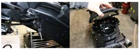
2. Identify and label the left and right hand turn signal connectors. Un plug the turn signal connectors after they are labeled. Un plug the OEM plate light connector.
