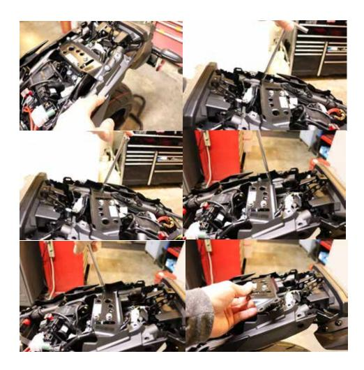
6. Cut the plastic zip tie used to hold the wire loom in place. Move the wires around to expose the nuts holding the fender in place. Remove the stock fender nuts and guide the wires through the center hole to complete the removal of the stock fender.
