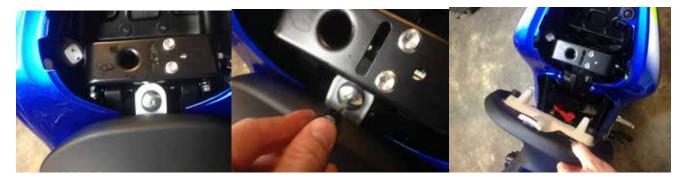
In order to remove the stock fender, the turn signal and plate light connectors will need to be unplugged. The connectors are located in the right side tail section. In order to un plug the connectors, the right side tail section body work will need to be removed.
