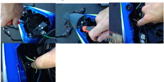
5. Remove the right side tail section by un snapping and sliding the tail section bodywork toward the front of the bike.
