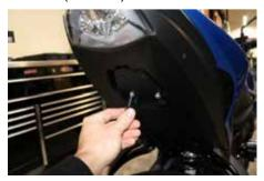
10. Mount the DMP license plate bracket using the two 6x1.0x16 button head bolts and two 6x12 (smaller) washers.
