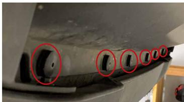
2. Using a trim removal tool, remove the eight push rivets along the front of the splash guard. We recommend prying on both accessible sides of the push rivets at the same time due to their large size.
