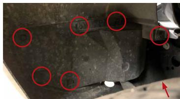
3. Remove the plastic fog light covers. To do so, use a 7mm socket and ratchet to remove the seven screws shown in the picture to the left.
