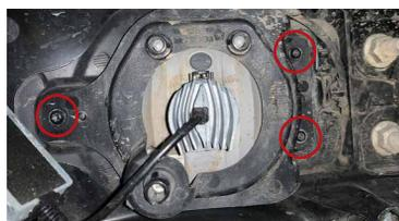
4. Remove the factory fog light assembly. Use a T20 Torx driver to remove the three screws. We recommend using hand tools to reduce the chance of thread stripping or heating of the plastic that may occur with power tools.
