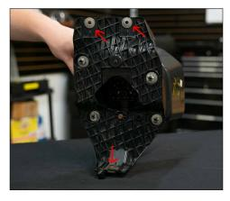
**11.** Reinstall the entire foglight bracket back onto the vehicle using the three 8mm bolts. Use the included wire adapters to connect the pod to the vehicle wiring harness. Test function. If the light does not turn on, try flipping the connector 180°.
