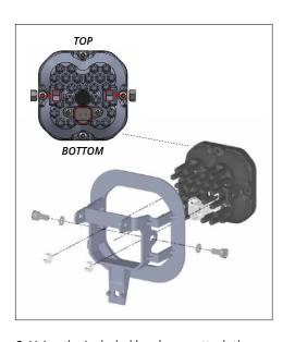
**6.** Using the included hardware, attach the Type SD bracket to the pod. See the diagram above and make sure the bracket is in the correct orientation. Tighten these bolts down all the way.
