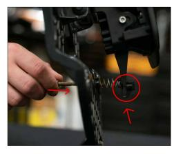
**8.** Reinstall the adjustment screw, spring, and plastic clip to the bottom of the bracket.
