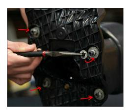
**10.** Reattach the metal retaining washers.
