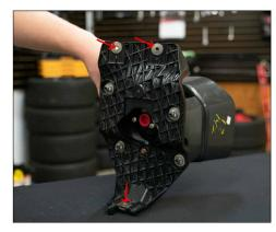
**2.** With the metal brace removed you can remove the entire foglight bracket assembly by removing the three 8mm bolts shown above.
