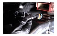
10. Reinstall the factory fog light bezel, by reinstalling the factory hardware. Plug the SS3 into the factory fog light harness using the included DT wire adapter. Test function. If the light does not turn on, try flipping the connector 180°.
