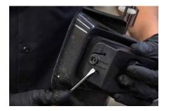
8. Remove the fog light housing from the bezel. To do so, remove the adjustment screw and spring from the fog light housing. Remove the factory fog light housing by prying up on the retainer clips holding it in place.
