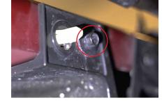
7. Remove the final 8mm bolt and loosen the plastic retaining clip to remove the fog light bezel from the vehicle.
