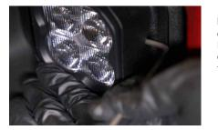
11. Adjust and aim the fog light according to your local and state laws. To adjust, loosen the screws on the sides of the bracket, aim, and re-tighten. In general, fog lamps should be angled slightly downwards to illuminate the area directly in front of the vehicle, below your headlamps.
