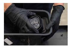
9. Install the SS3 bracket on to the factory bezel by flexing the retainer clips on the bezel as required.
