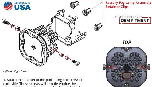
of your SS3 pods. Adjust the angle of the light in the bracket, then tighten down these screws. See diagrams above and to the right. Make sure the bracket is in the correct orientation.
