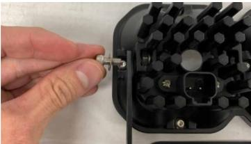
7. Attach the U-bracket to the pods using the included screws and washers. Hand tighten only.
