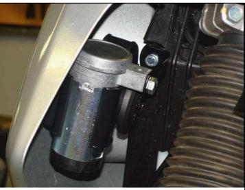
Mount the horn to the bracket using the hardware provided with the horn. Be sure to read all mounting instructions provided with the horn to ensure it is mounted at the right angle.
