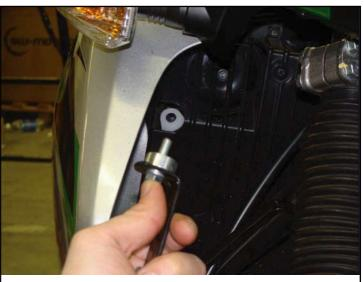
Attach the mounting bracket with the M6 screw provided. Place the 7mm spacer behind to the bracket.
