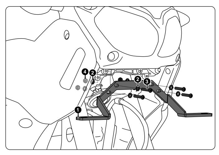
**Step One:** Use the supplied hardware to bolt the bracket to the four mounting points located under the headlight of your motorcycle.
