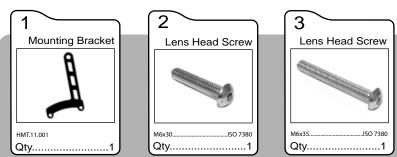
Step One: Remove the two bolts shown from your engine case, place the bracket and replace the bolts with included hardware. Be sure that the longer bolt goes in the hole closer to the tail of the bike.
