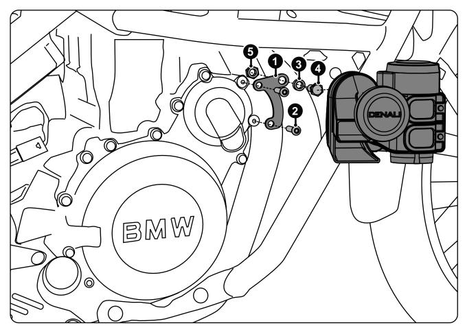
Step One: Using the supplied hardware mount the bracket to the motorcycle as illustrated above.
