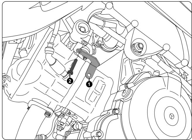
**Step One:** Remove the bolt from the engine mounting clamp located on the left hand side of the bike. Use the included M8 screw (#2) to bolt the horn mounting bracket (#1) to the clamp as illustrated above. Attach the horn to the mounting bracket.
