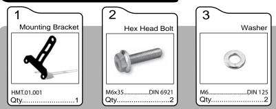
Step One: Remove the two OEM bolt from the right side engine case as illustrated above. Use the bolts (#2) and washers (#3) to bolt the bracket (#1) to the motorcycle. Bolt the horn to the mounting bracket using the hardware that was supplied with the horn.
