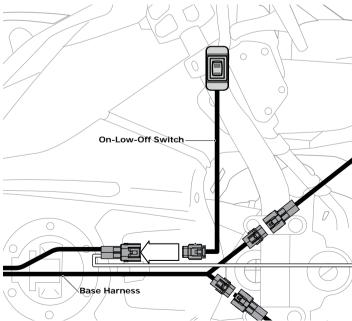
lights, separate from the vehicles OEM lighting system. This eradicates the issues presented by vehicles that do not provide and a clean 12v high beam trigger signal. This switch is also a great option for those who
