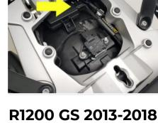
Connect to the RDC connector located under the passenger seat at the rear of the opening..
