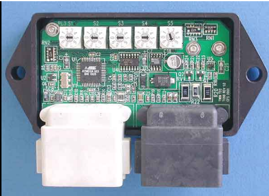
Twin Tec TC88 Ignition Module
