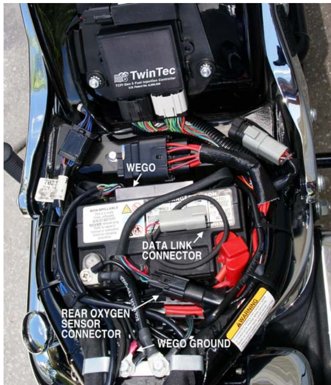
Figure 23 - Typical Softail® Installation
