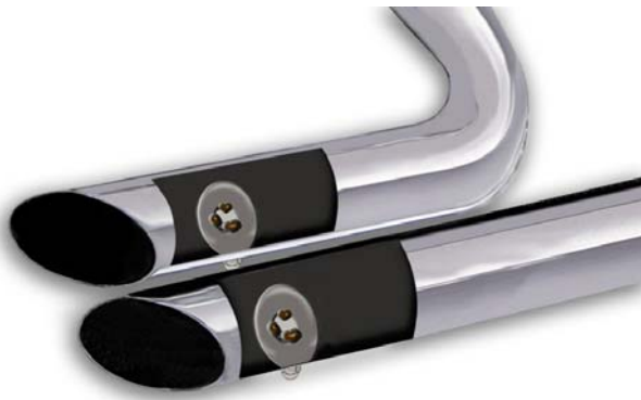
Figure 1 – Exhaust Mod to Reduce Reversion
