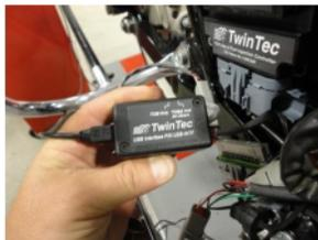
15. Plug the USB interface into the four terminal data link connector coming from the TCFI harness and the USB cable into your computer. Make sure the switch on the USB interface is set to the TC88A and All Others position.
