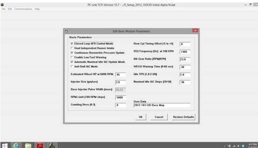
21. The Edit Basic Module Parameters window will automatically pop up. For most applications, you can use the default settings. **Verify that Estimated Wheel HP, Injector Size, RPM Limit, and VSS Frequency are correct for your application.** Refer to the TCFI instructions for details. Call our tech support if you need help.
