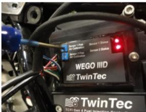
13. After two minutes, use a small screwdriver to slowly turn each trim pot screw on the WEGO clockwise until the corresponding LED just starts flashing. This will calibrate your oxygen sensors. Turn off the motorcycle. After the sensors cool down, you can install them into the exhaust. Complete install of the WEGO, and secure any wiring appropriately.
