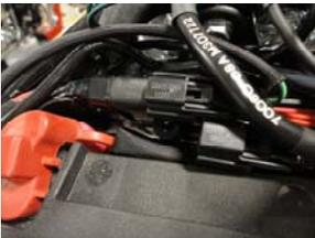
10. Locate the front and rear factory oxygen sensor harnesses. Disconnect the factory oxygen sensors and plug the mating connectors from the WEGO into the factory harnesses.
