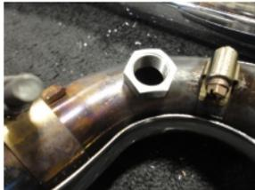
9. Weld a bung into each pipe. After the pipe has cooled, use an 18x1.5mm tap (standard spark plug tap available at most parts stores) to clean the threads. Reinstall the exhaust system.
