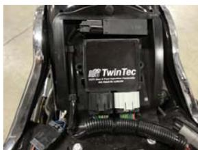
4. Remove the factory ECM and install the TCFI controller. Make sure that the two connectors are properly mated to the TCFI.
