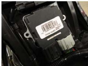
2. Make note of the motorcycle VIN and odometer reading (miles or kilometers). These values must be correct and will be entered in the software later. Remove seat, saddlebags, side cover, and other items to gain access to the factory ECM and data link connector.
