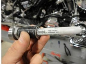
6. Skip to step 10 for exhausts with 18mm oxygen sensor bungs in the exhaust pipes. Carefully plan the sensor location approximately 2-6" from the exhaust port. Use a permanent marker to locate the position where you will drill a hole for your oxygen sensor bungs. If you have free flowing mufflers, try to locate the bungs as close to the exhaust port as possible.
