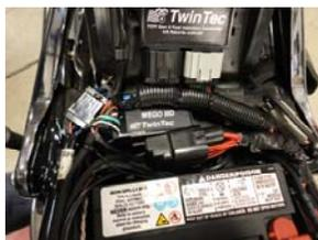
5. Install the WEGO IIID unit in an appropriate location. You will need access to the trimpot screws for initial setup, so do not permanently mount the unit at this time. Route the harnesses for the front (2 long) and rear (2 short) oxygen sensors to their respective locations. Final routing and securing can be done after the sensors are installed in the exhaust pipes.
