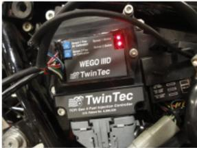
12. To calibrate the sensors, leave the off/run switch off. Turn the ignition switch on. This will power up the WEGO. The two red LEDs on the WEGO should illuminate. Use a small screwdriver to turn the two trimpot screws gently counter-clockwise until they stop. Let the sensors warm up for two minutes. Caution: the sensors will get hot.
