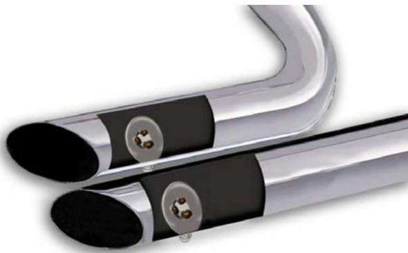
Figure 1 – Exhaust Mod to Reduce Reversion
