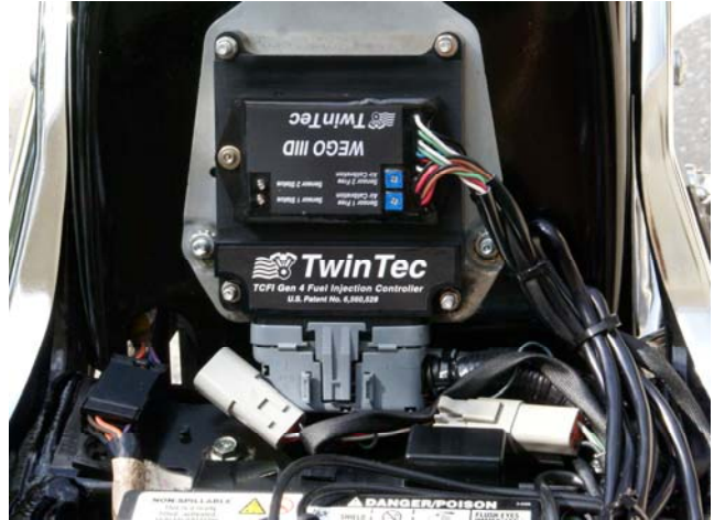
Figure 23 - Typical Twin-Cam Installation with WEGO IIID Mounted on Top of TCFI Unit
