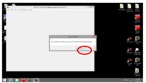
24. Turn the ignition switch on and the off/run switch to run. Open the TCFI Log software. Click YES.
