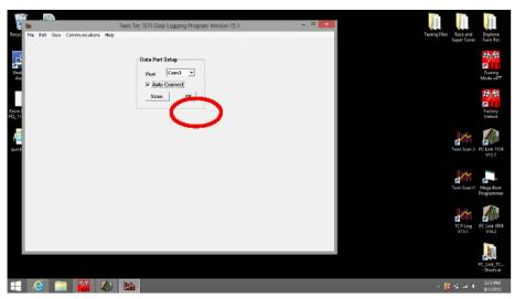
25. Click scan. The software should automatically locate and assign the COM port. COM port assignment will depend on your computer. Select Auto Connect and click OK.
