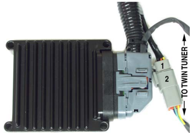
Figure 5 – Completed Wiring at ECM
