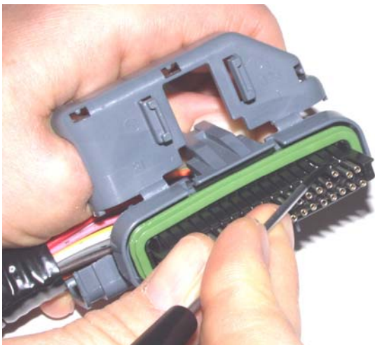
Figure 4 – ECM Connector Terminal Removal
