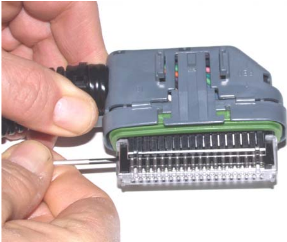
Figure 3 – ECM Connector Disassembly
