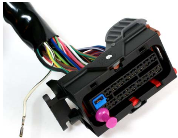
Figure 3 – ECM Connector Terminal Removal
