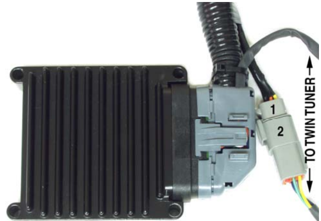
Figure 5 – Completed Wiring at ECM
