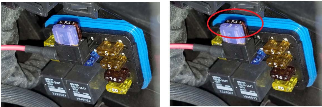
Figure 19C – SYSTEM 7.5A Fuse tap connection for switched uninterrupted power on 2018
