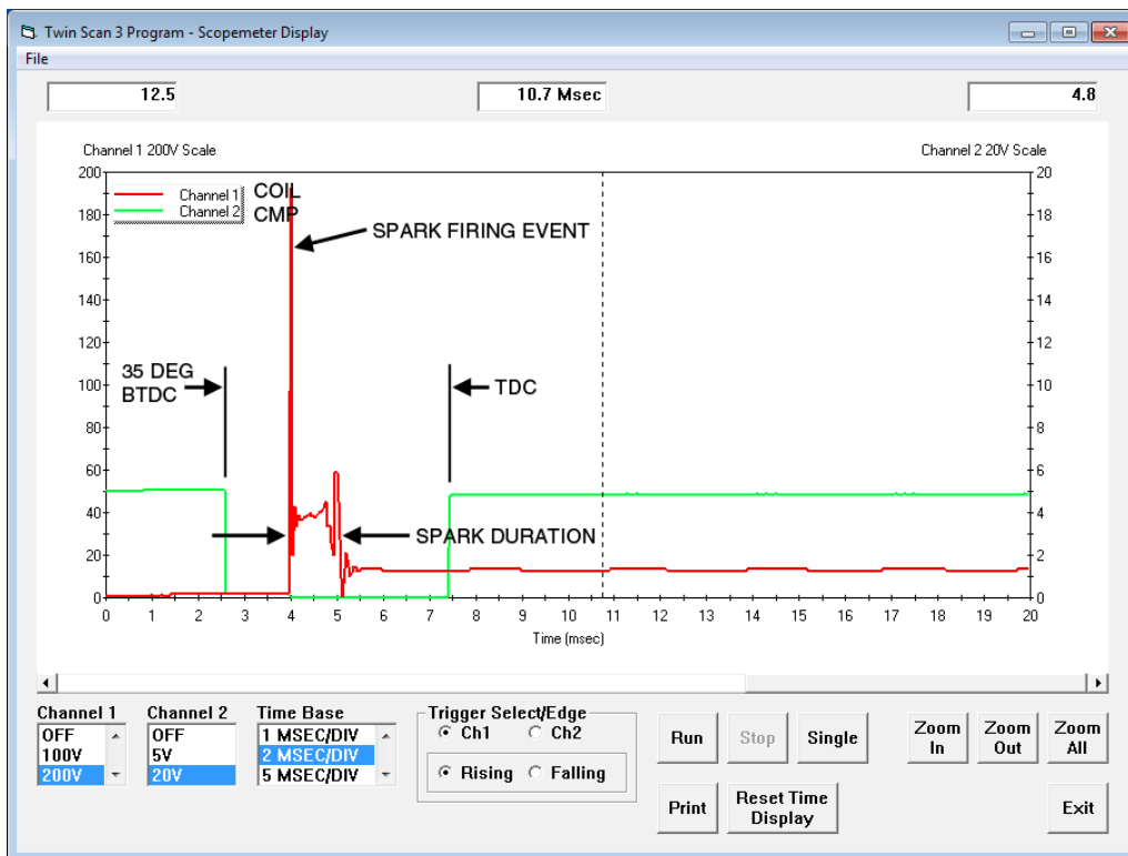
Figure 4 – Evo Coil and CMP Sensor Waveforms
