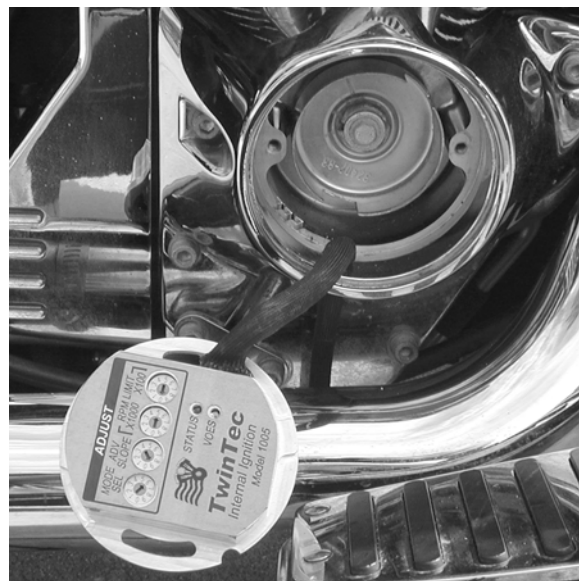
Figure 1 - Feeding Harness Thru Exit Hole
