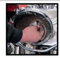
2. Now thread an 18" length of 16-gauge wire though the grommet and out of the left side of the triple tree covers.
