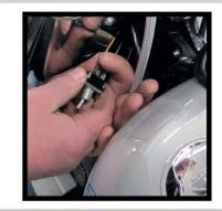
4. Pull the yellow wire (the one that is activated when this switch is turned on) from the back of the switch.
