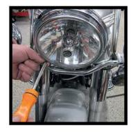
2. Then remove the three screws that hold the beauty ring to the headlight bucket using a #2 Phillips screwdriver. Lay this ring and these screws aside for reinstallation later on.
