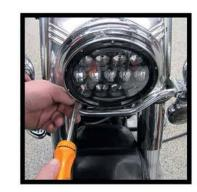
6. Now reinstall the stock beauty ring using the three stock screws and a #2 Phillips screwdriver.
