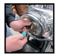
4. You can now just plug the new Cyron LED headlight to the bike's stock headlight harness. As for the red wire, which powers the daytime running lights, you can leave it as is.
