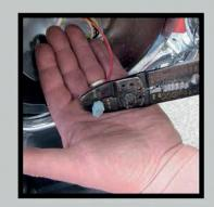
9. Cut the wire you installed so about 7" of it is in the headlight bucket and bare about 3/8" of wire. Then install a female blade connector on the wire and a male connector onto the short red wire on the new LED headlight plug.
