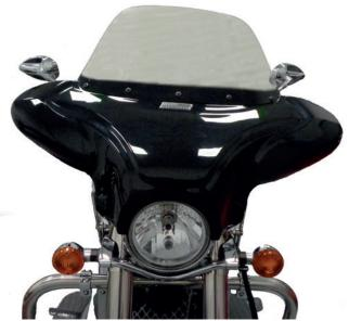
It would be convinient to retight the windshield screws, specially the ones that are fi xed to the motorcycle, whenever you maintain the vehicle.
