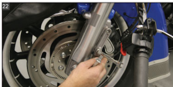
22 Loosen the brake hardware and remove both calipers.
