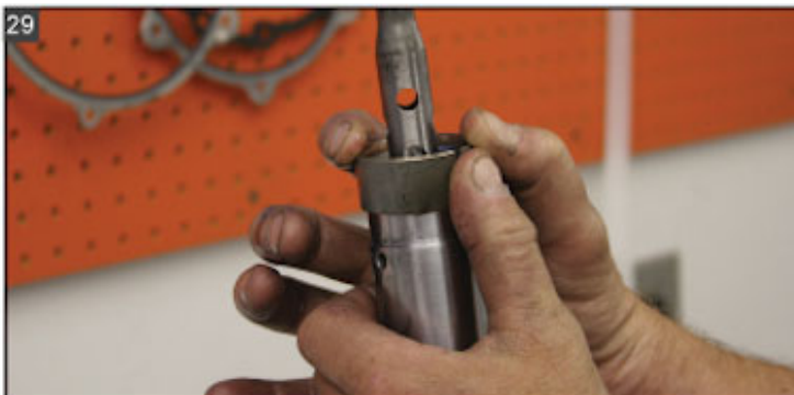
Install new seals and bushings as needed while reassembling the fork tubes.
