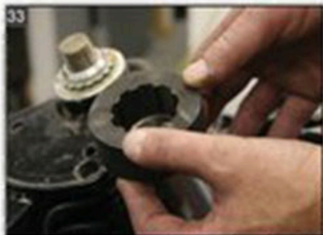
33 Install the rubber fork-stop donuts onto the tubes.
