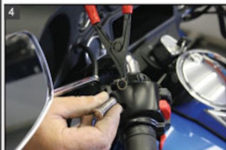
Disconnect the clutch cable to enable the removal of the fairing.
