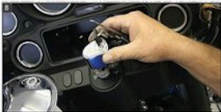
8 Remove the locking ignition switch assembly; this requires the use of the ignition key.
