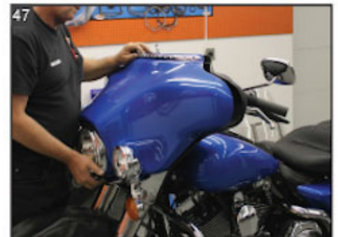
47 Reconnect and check all of the remaining wires, then install the fairing and windshield.
