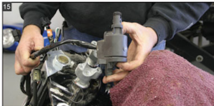
15 Unbolt the ignition switch and set it aside.
