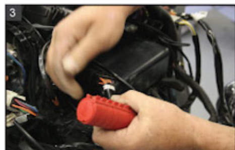
The inner fairing must come off. Label all of the wires and plugs to save you some trouble later.
