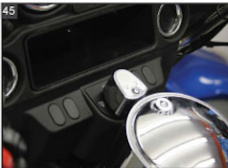
45 Install the ignition switch housing.
