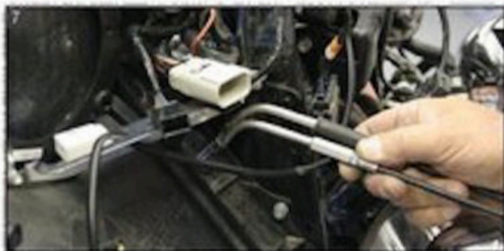
7 Pull the cables through this hole to the front side of the inner fairing.
