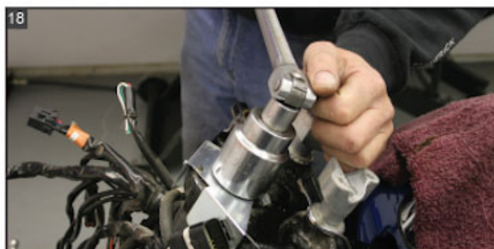
18 Loosen and remove the fork stem nut.
