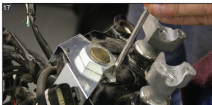
17 Bend the fork stem nut lock tab down and out of the way.
