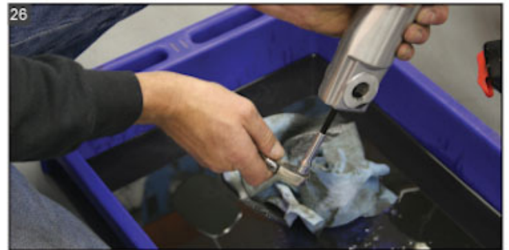
Pull the allen-head bolt out of the lower fork leg assembly and allow the fork leg to drain.
