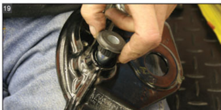
19 Wiggle the riser mounts out of the stock triple clamp.
