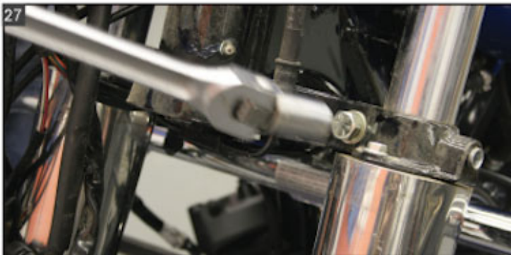
Loosen the pinch bolt to allow the fork legs to come out of the lower triple clamp.
