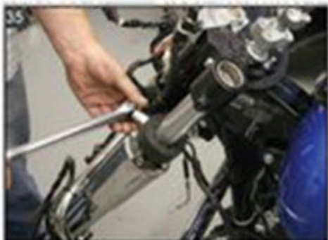
35 Make sure the tubes are flush with the top triple clamp then tighten the pinch bolts. Add fork fluid now.
