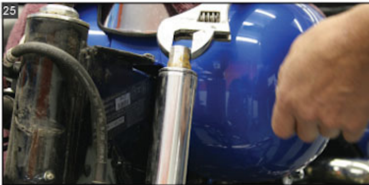
Loosen and remove the fork caps on both sides.
