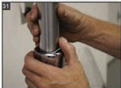
31 Install the snap ring making sure it is seated completely.
