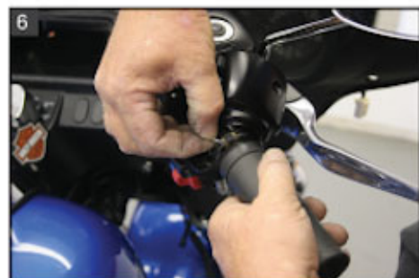
Remove the throttle cable barrels on the right grip to allow the cable to be separated from the throttle grip.
