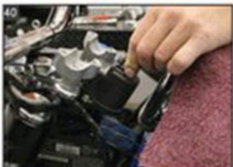
40 Bolt the ignition switch into place on top of the new triple clamp.
