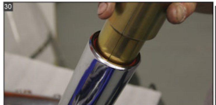
Use a slide tool to correctly seat the seal so the retaining ring can be installed into the groove in the slider.
