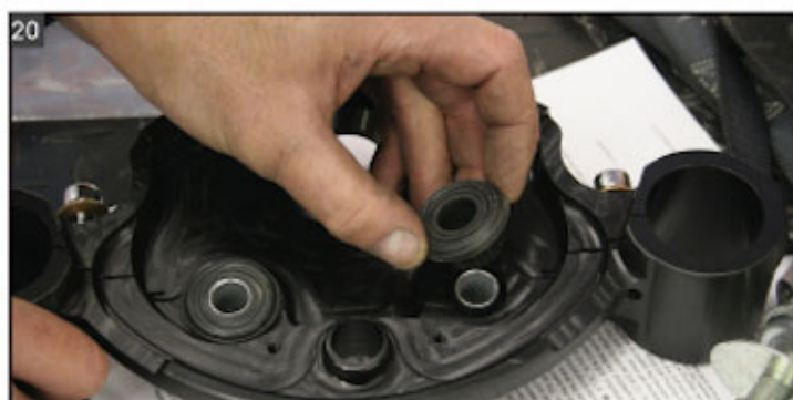
20 Install the riser mounts into the CCE top triple tree.
