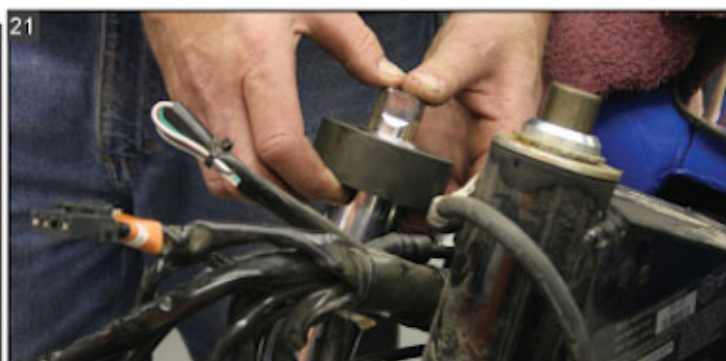
21 Pull the rubber fork stop donuts off of the fork tube.
