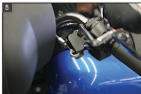
Push the cable through to the front of the inner fairing.
