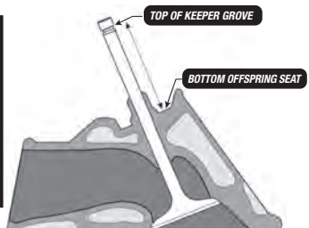
Diagram 1. Calculating Installed Spring Height
