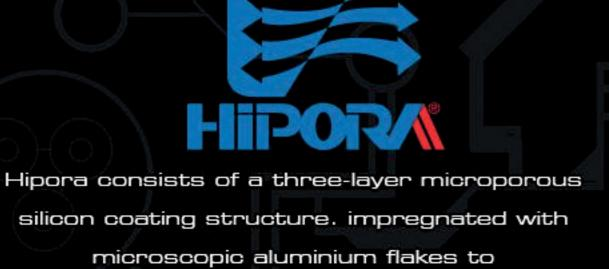
microscopic aluminium flakes to enhance heat retention characteristics. The first layer prevents water penetration and peeling. The second layer achieves moisture permeability and resistance to water penetration. The third layer increase water resistance.
