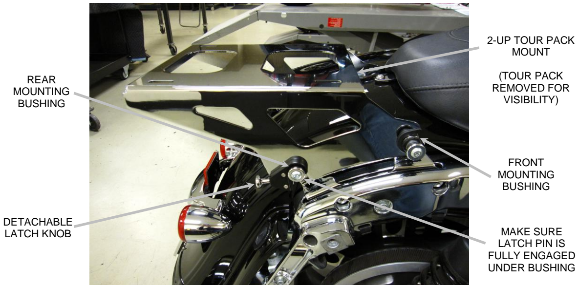
FIGURE 2, TOUR PACK MOUNT INSTALLED
