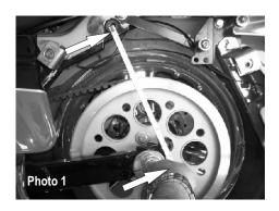
Do Not complete your Slammer Shock installation until you have checked to be sure you have adequate Tire / Fender clearance.
