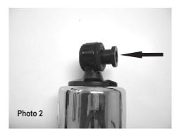
Install a shouldered sleeve as shown into each mounting eye of both shocks
