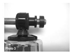
On 1991 - Later Sportsters also use one additional spacer in conjunction with the shouldered sleeve to provide sufficient space between the shocks and the Frame / Swing arm.
