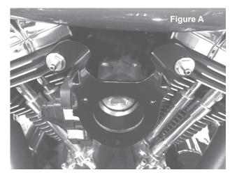
■ Install welded backing plate (11) using the 3 ¼-20 socket cap screws (2) into corresponding throttle body threaded holes as shown in FIG B. Torque ¼-20 socket cap screws to 40-60 In-lbs.
