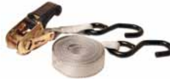
TD304-1 Ratchet tie-down • Easy to use: attach and pump handle • Vise-like gripping power • Bully tough-cut and abrasion resistant • 15' length / 5000lbs break strength / 1666lbs work load limit
