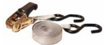
TD400-1 Cambuckle • Easy to use: attach and pump handle • Vise-like gripping power • Bully tough-cut and abrasion resistant • 15' length / 400lbs break strength / 135lbs work load limit
