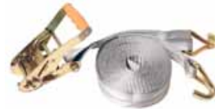
TD501-1 Ratchet tie-down • Easy to use: attach and pump handle • Vise-like gripping power • Bully tough-cut and abrasion resistant • 27' length / 10000lbs break strength / 3300lbs work load limit
