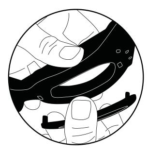
The clips on the bezel of the lenses on either side of the frame should release from the frame.
