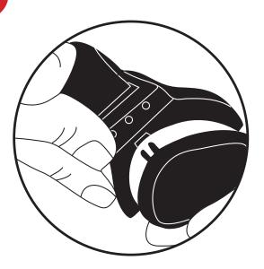
Push outside clip on lens bezel into the hole on the frame. Then push the other clip into the corresponding hole on the frame.
