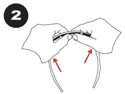
Align the two tabson each end of the foam with the two slits on either side of the frame. Push the foam into the slits on frame until secure.
