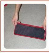
Remove the larger dirt by shaking or tapping your filter gently onto a clean surface. DO NOT use compressed air which may damage the filtering element.
