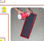
Distribute the BMC detergent on the filter. Allow to absorb for about 10 minutes. DO NOT use caustic products such as petrol or oil. USE ONLY BMC DETERGENT.
