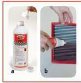
Remove the original top from the regenerating fluid bottle. Make a small hole in the spout dispenser and screw onto the bottle. For correct oiling we recommend passing the regenerating fluid twice over every pleat on both sides of the filter.
