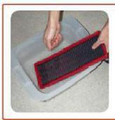
Wash your filter in cold water. Rinse well ensuring that dirt does not enter the filter pleats. DO NOT use high-pressure water.
