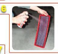
The oiling procedure using the aerosol spray. Hold the spray 15 cm from the filter and spray the complete surface. Repeat the operation on both sides of the filter.
