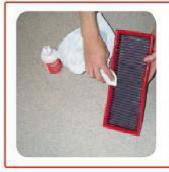
Allow the oil to absorb on a level surface for around 30 minutes. Remove any excess oil on the rubber and check that the filtering element is homogeneously red (Picture 7). If not, repeat the oiling process described Previously. After oiling the filter is ready to be reinstalled.
