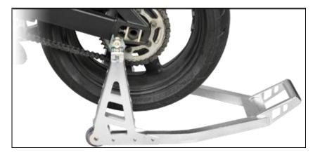
And, if you use a rear stand, we recommend the use of BikeMaster Spools on bikes that have the threaded adaptors fitted from the factory. These spools allow you to use the V-Saddles, which provide a more secure lift for your machine (as shown above).
