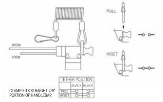
Normally-closed kill switches are used to complete a circuit when the lanyard clip is installed. When the lanyard clip is removed, the circuit is opened, disabling it.
