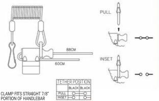
Normally-open kill switches are used to create an open circuit when the lanyard clip is installed. When the lanyard clip is removed, the circuit completes a ground, stalling the machine.
