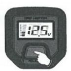
In volt meter screen, press the button once to enter the quick heat up mode:
