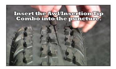
2. Insert the Awl/Insertion Tip into the puncture of the tire.
