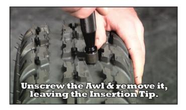
3. Unscrew the Awl and remove it, leaving the Insertion Tip in tire. Apply the rubber cement to the rubber plug. (Be sure to use enough cement to lubricate the plug)
