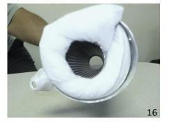
**Step 8: (Fig 17)** If the packing pillow begins to bunch up, you may need to use a tire iron, ruler or other sturdy object to push down the bunched up packing. Be sure to correctly align the core so that it fits over the inlet cap at the bottom of the muffler.
