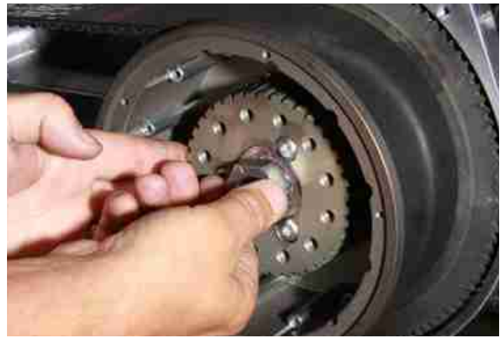
Install clutch hub nut supplied with kit, left hand thread.
