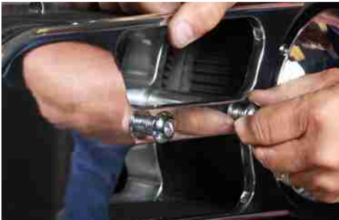
Install side guard using the 2 ea 1/2-13 x 1 SH BH cap screws.
