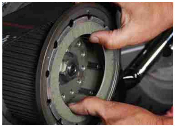
Install clutch fiber, then alternate steel and fiber ending with a steel behind the pressure plate. As shown in the enclosed DVD
