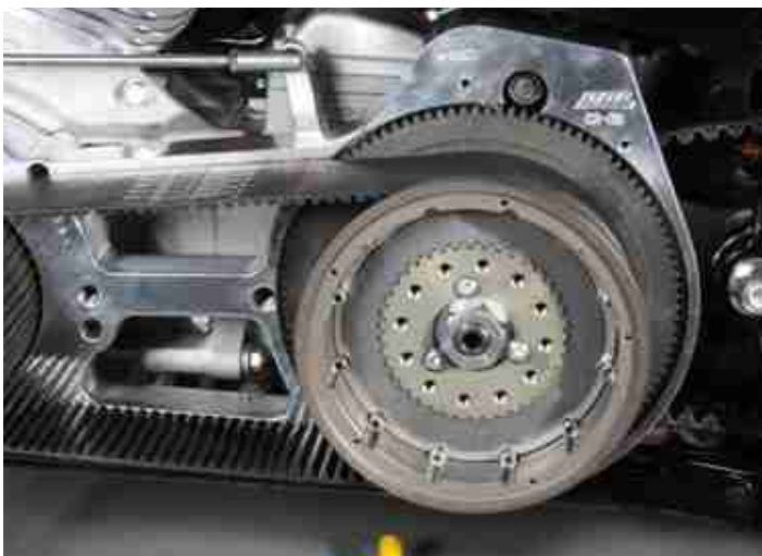
Completed clutch pack installation.
