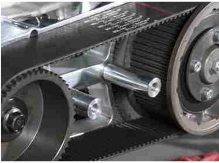
Standoffs shown installed into motorplate.
