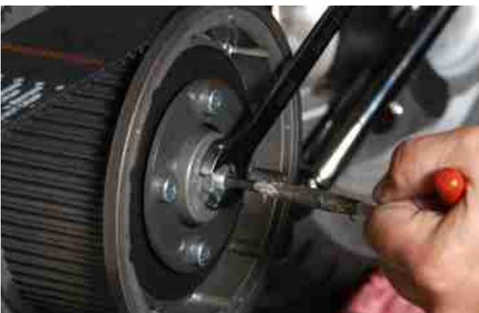
Install clutch adjusting screw, adjust clutch and tighten jam nut. As shown in the enclosed DVD.
