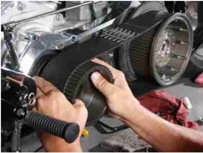
Install front pulley and belt, be sure that the writing on belt is facing you.
