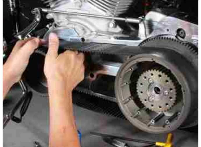
Be sure belt and pulleys are seated properly.
