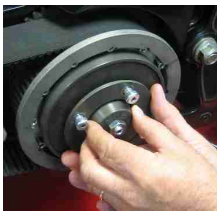
While firmly holding assembly on clutch basket, locate holes in the clutch hub and screw the shoulder bolts in.
