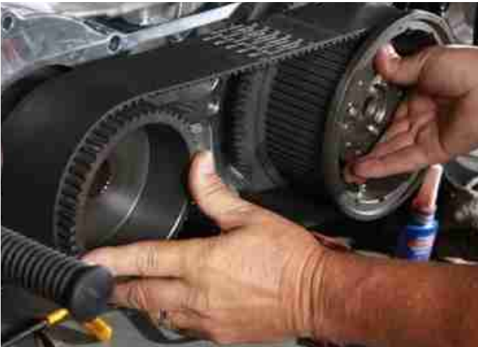
Install both pulleys and belt to check for fitment.
