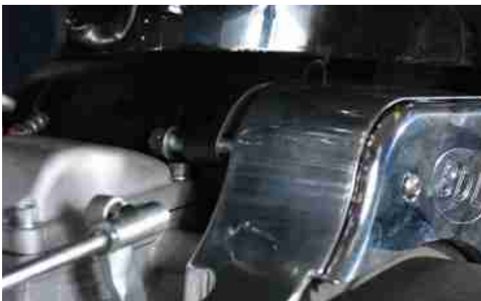
Re-tighten starter to motorplate from opposite side of bike.
