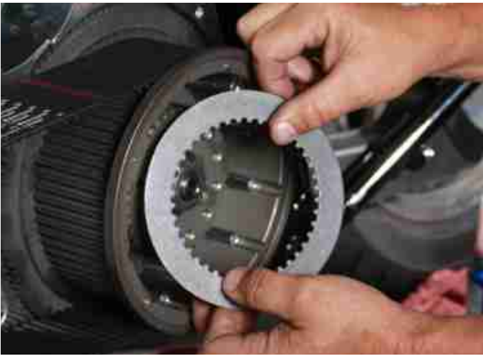
Install thick steel first, (.120" thick) As shown in the enclosed DVD
