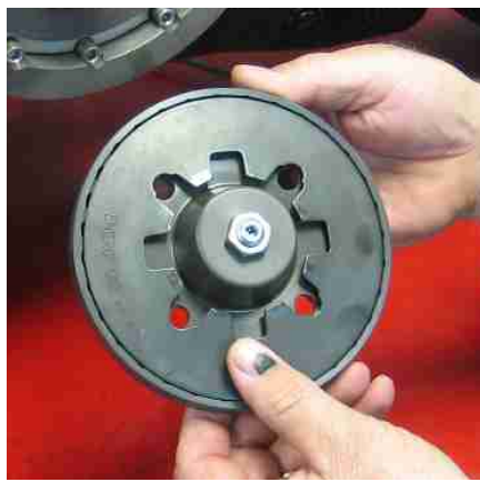
Place BDL diaphragm over ball bearings on pressure plate.
