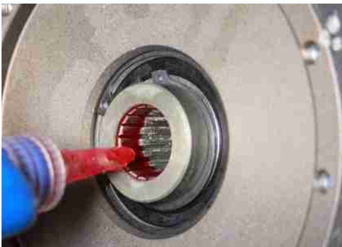
Apply red Loctite® to spline area on the inside of splined clutch hub from back side of clutch basket.
