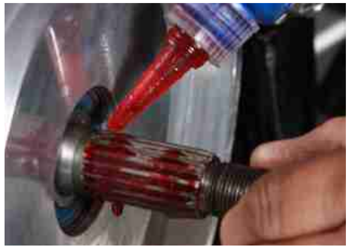
Apply red Loctite® to spline area of mainshaft
