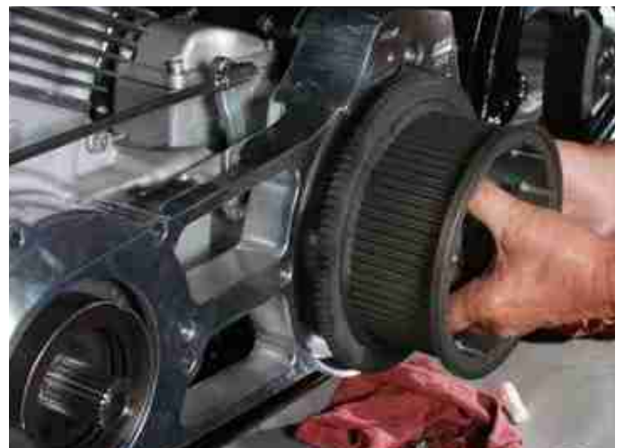
Install clutch basket assembly onto mainshaft.
