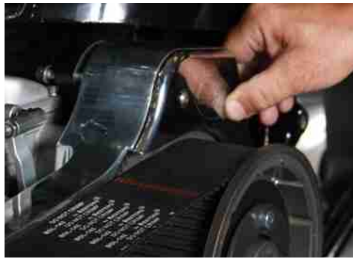
Install starter housing using the 2ea 1/4-20 x 1/2 SH BH cap screws.
