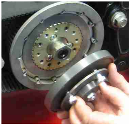
Holding assembly with pressure against the diaphragm so that the ball bearings are secured, place assembly on to clutch basket.
