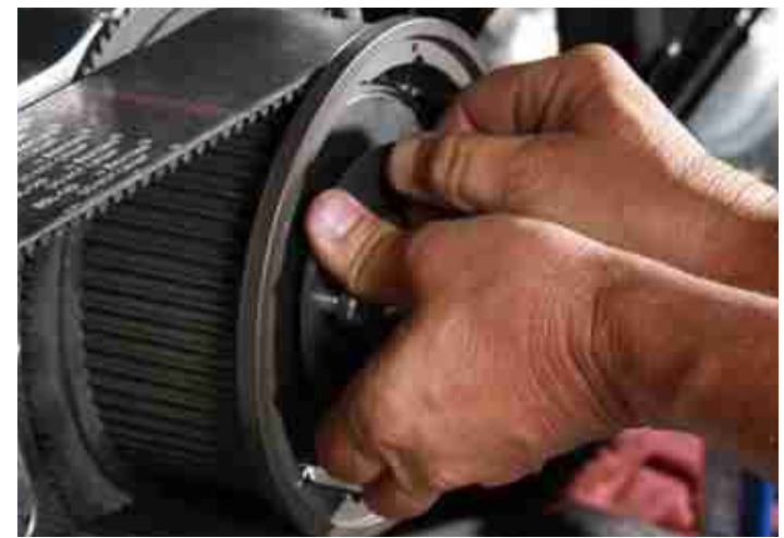
Install ball bearing lock up as shown on the last page of this guide, and in the enclosed DVD.
