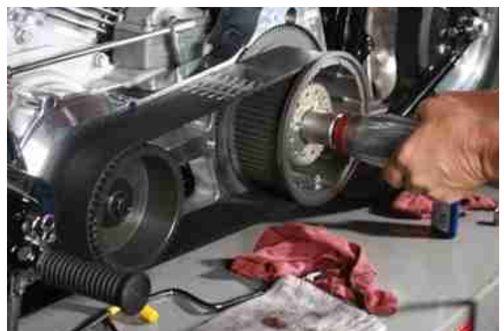
Tighten clutch hub nut and torque to Harley specs.
