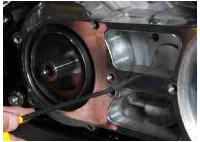
Install motorplate using the 5ea 5/16-18 x 1-1/2 shoulder bolts and 4ea 1/4-20 x 1-1/2 shoulder bolts supplied with kit.
