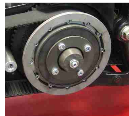
Tighten shoulder bolts down to approx. 25 TO 30 foot pounds.
